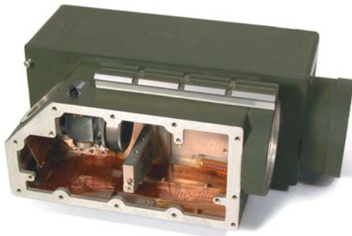
After: The package is neat, lightweight, and less susceptible to connection failure.
