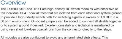
All modules are also configured to avoid any unterminated stub effects. This improves overall signal integrity and allows for high frequency matrix designs or large multiplexer configurations while preserving bandwidth and maintaining low VSWR. The front panel utilizes two high-density, 26-pin coaxial connectors designed for high reliability and low insertion loss.
