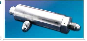
The Kulite BMD/BMDE-1100 Series pressure transducers are designed for the measurement of pressure drop across air and oil filters, engine torque and similar applications. Available either unamplified (100mV output) or amplified (5 volt output), these units are all stainless steel construction with weld sealing offering maximum accuracy and performance for industrial and aircraft applications.
