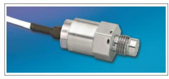
Incorporation of a Kulite proprietary electronics module within the main body of this product allows for operation from an unregulated power supply ranging from 12  $\pm$  4VDC or 28  $\pm$  4VDC with reverse polarity protection available upon request. The result is a stable, microprocessor corrected 0 to 5 VDC output signal.
