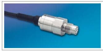
diaphragm is used as a force collector. Force is transferred to a solid-state piezoresistive sensing element via thin intervening film of non-compressible silicone oil. This sensing sub-assembly is protected from mechanical damage by a protective screen, which has been shown to have minimal influence of the frequency response of the sensor. Incorporation of Kulite proprietary high temperature 365°F (185°C)
