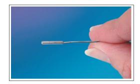
The XCL-062 design features Kulite's patented leadless technology. This allows for a very rugged package suited for probes, pressure rakes and other similar test set ups. This transducer is well suited for both dynamic and static pressure measurements in benign or harsh environments.
