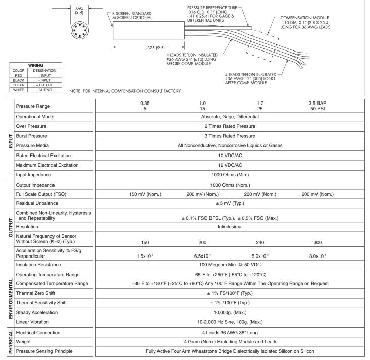
Note: Custom pressure ranges, accuracies and mechanical configurations available. Dimensions are in inches. Dimensions in parenthesis are in millimeters. Continuous development and refinement of our products may result in specification changes without notice - all dimensions nominal. (L)
