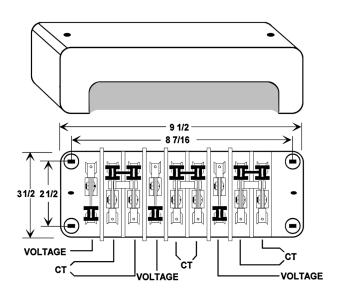
SWITCH DIMENSIONS 9 1/2" X 3 1/2" X 2 3/4" COVER DIMENSIONS 10 1/8" X 4 5/8" X 3 1/8"
