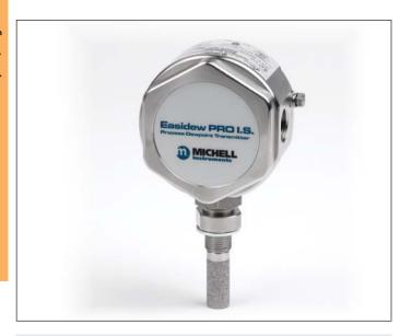
The Easidew PRO I.S. is a rugged intrinsically safe 2-wire dewpoint transmitter for trace moisture measurement in liquids and gases. It is certified for use in IS Class 1 Div 1 Groups A,B,C and D, Ex II 1G EX ia IIC T4 and I.S. I 1 ABCD T4 (Ta = +60°C) hazardous area locations.
