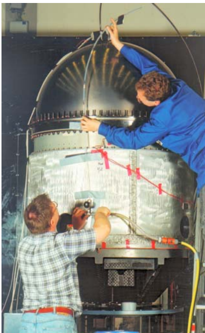
Strain gage measurements on an ATV (Automatic Transport Vehicle) tank at EADS Deutschland GmbH, Ottobrunn/Germany
