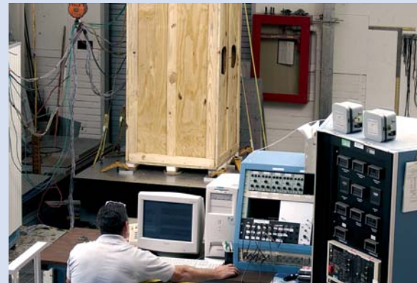
Earthquake simulation at Lucent Technologies, Whippany/New Jersey
