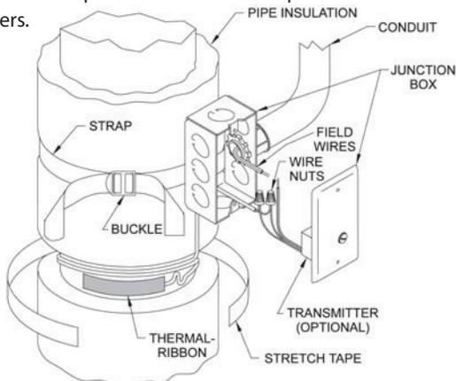
Note: Tape the Thermal-Ribbon in place beneath a layer of insulation.
