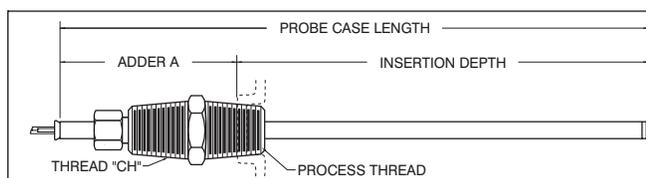
To determine the ideal probe length add the insertion depth to the adder A for the fitting you will use.
