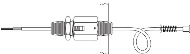
When selecting the FG1015 or FG3015 for use with silicone filled cable use the grommet hole size from the tables.
