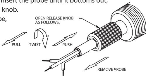
Spring pressure holds the probe tip in contact with the measuring surface for faster response and more reliable measurements. Many models feature a rubber O-ring that doesn't crimp the probe but prevents oil leakage to 50 psi (3.4 bar) at up to 260°C. High temperature models are usable to 450°C. Nylon versions provide electrical insulation.
