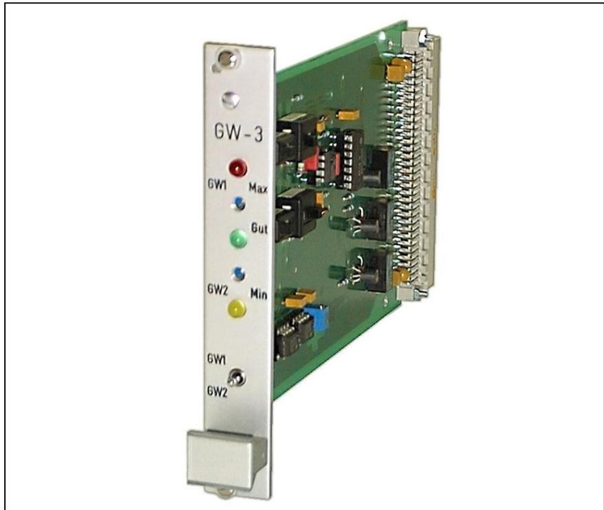
If the GW-plug-in unit is being used in connection with a VVE-DR or a VVE-DMS plug-in unit, the output signal can be adapted for an indicator through the VVE-plug-in's; here-with the measuring values and the limit values are being displayed dimension-equitable.
