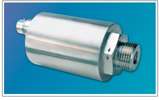
This transducer is a drop-in replacement for older type electromechanical synchro transducers (transmitters). It incorporates the Kulite patented Silicon on Insulator (SOI) piezoresistive sensors and custom electronics to produce a transducer Fit, Form and Function equivalent to the older parts, but with significant improvements versus the electromechanical devices.
