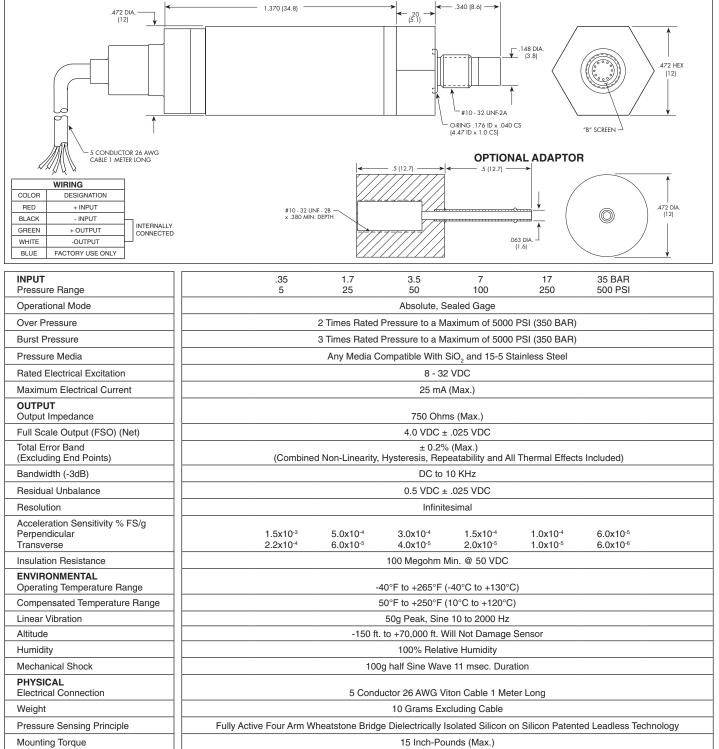
Note: Custom pressure ranges, accuracies and mechanical configurations available. Dimensions are in inches. Dimensions in parenthesis are in millimeters.
