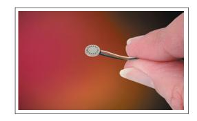
The LLHT Series features Kulite's Patented Leadless Technology and demonstrates Kulite's ability to provide pressure transducers suited for adaptation into custom packages. These devices can be integrated into various test articles such as fan blades, engine nozzles of various types, etc. The features of these transducers include small foot print, high natural frequency, extreme resistance to vibration and shock, and wide temperature range.
