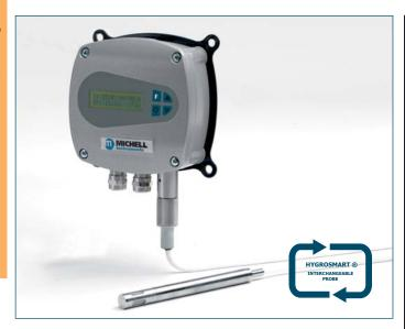
The WR293 relative humidity transmitter uses the Hygrosmart module, integrated in the interchangeable probe. This device can be used in high-temperature applications due to the remote measurement element and its small overall size. The interchangeable probe allows for simple recalibration and lower maintenance costs.
